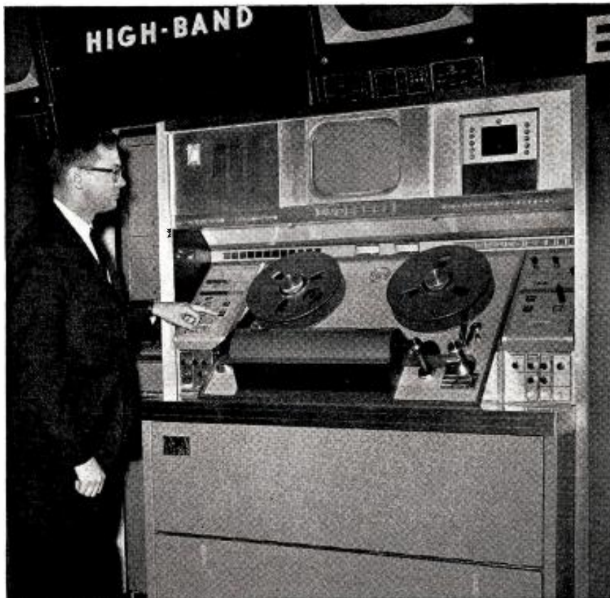
Designed, built and factory tested as a completely integrated color tape system, the TR-70 offers better performance than previous high-band machines.
