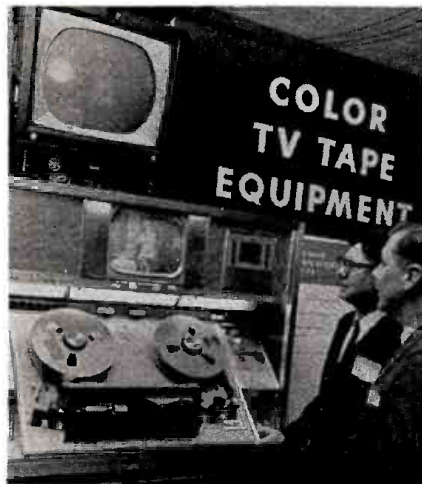
Robert J. Kreis (l), WLWC(TV) Columbus, Ohio, discusses RCA's new high band color video-tape recorder, the TR-70, with manufacturer's H. H. Klerx.
