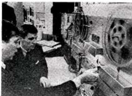
Harwald Co.'s film inspection and editing machine is demonstrated by company's Bill Stelcher (l), for Rex Marx, WBAY-TV Green Bay, Wis.
